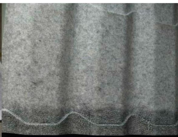
Graphic 11: Roofing tile with thermal sealing
